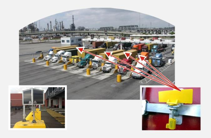
This system, built on smart UHF RFID reading units and passive (battery-free) RFID UHF seals - named e-SEALS, is able to identify and monitor in a reliable and secure way trucks, trailers, and containers.
