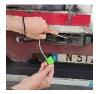
Insert the cable into the holes to be sealed.
