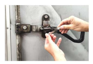
Insert the tail of the seal in the back hole of the seal head.
