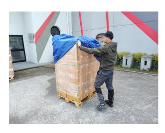
Place the pallet cover "Bologna" on the pallet to be covered, and slide it along the four sides.
