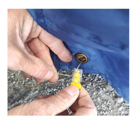
Nylon pallet covers may protect any product at any attempts at tampering since they can be sealed with a wire security seals — e.g. Twistseal with 500mm sealing wire pre-insert.
