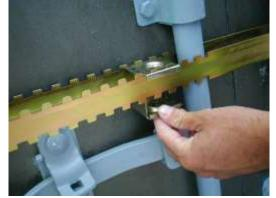
2.) ... insert the second joint exactly in connection with the first one.
