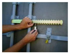
4.) ... Insert the bolt lock and set off the locking mechanism. FROM THIS POINT FORWARD, THERE IS NO POSSIBILITY OF TAMPERING.
