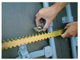
1.) Position NEW FORKSEAL between the central barriers of the container and insert the first joint the closest possible to the barrier...
