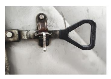
By doing so the seal is locked. The only way to open it is to break it.
